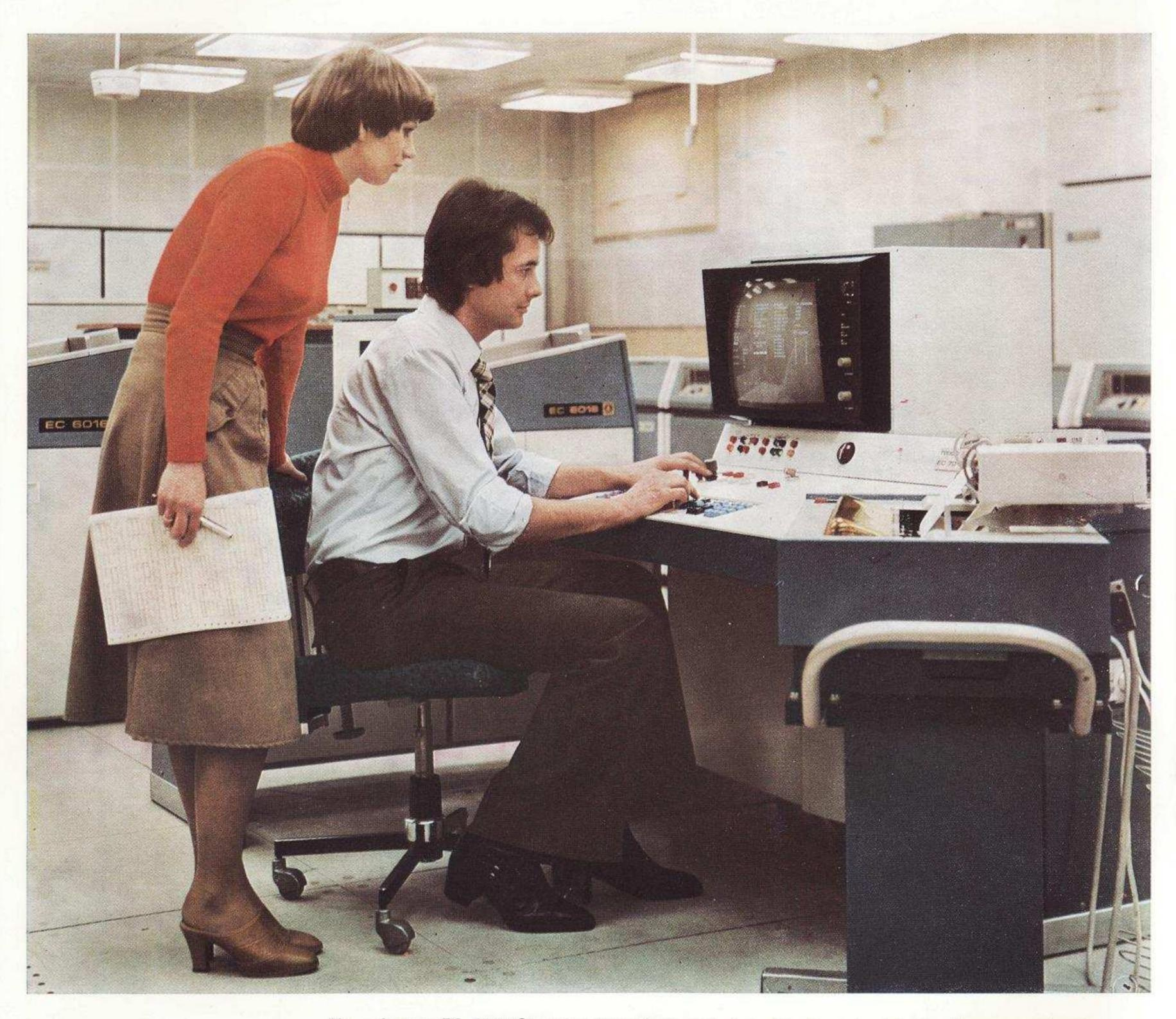
The robotron EC 7069 Operator Console is a device of independent design for communication between operator and operating system and between maintenance personnel and computer. It contains all technical means for operation and display as required for this communication.
